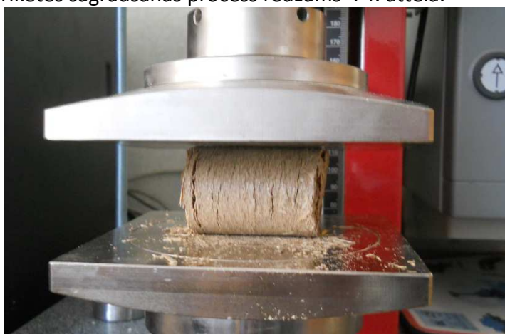
74. att. Brieketes sagraušanas process
