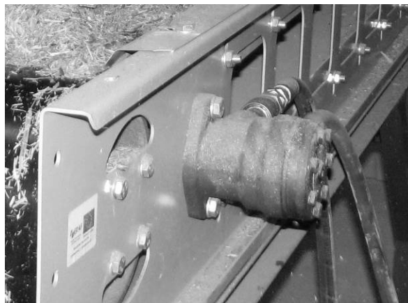
Fig. 4. Hydraulic drive of feeder
