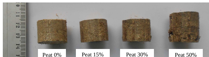
Fig. 8. Common reed and peat mixture briquettes Notes: Common reed particles from grinding screen opening size 6 mm.
