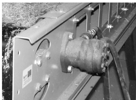
Fig. 4. Hydraulic drive of feeder
