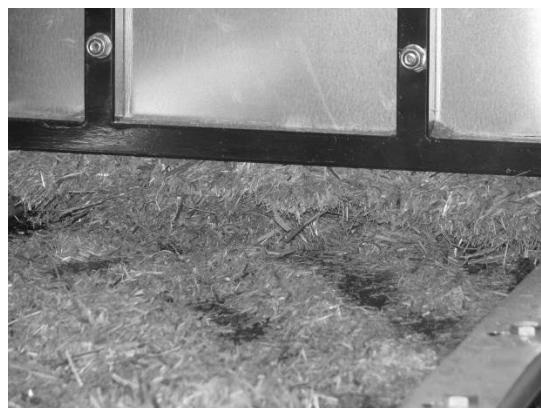
Fig. 13. Jam of chopped biomass
